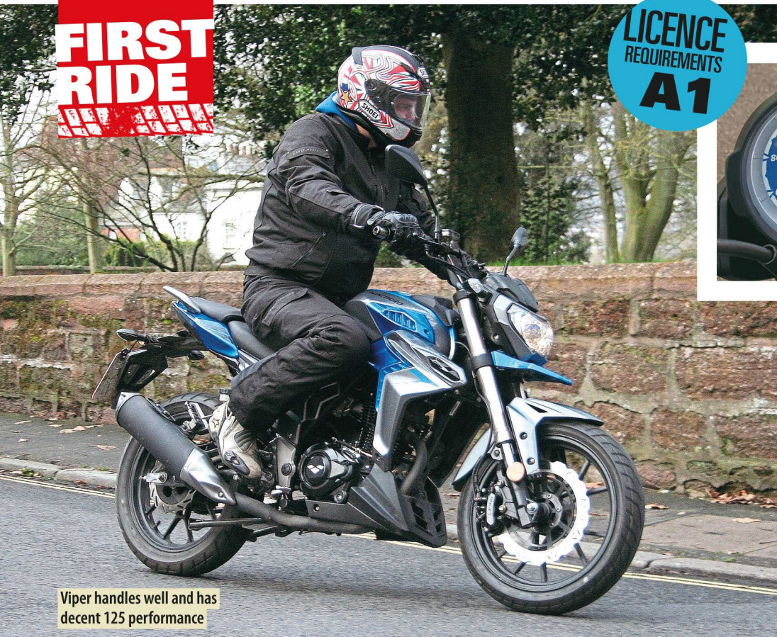
Three-piston front caliper allows for linked brakes
