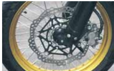
296mm disc and twin-pot caliper make CRF's brakes the best of the bunch
