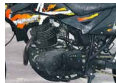
Pulse has an air-cooled single, fuelled by a carb. It vibrates but has charm
