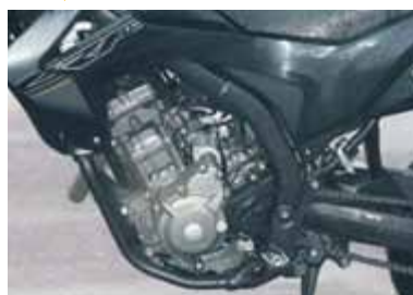
Honda's proven CBR250 engine nestles between the CRF's steel cradle frame
