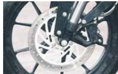
Caliper is made by ByBre – which is actually short for 'By Brembo'
