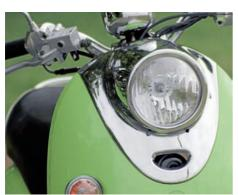
on it, but Mau complained that his knees were hitting the handlebars. The scooter has a nice short wheelbase which makes it feel a bit like a Piaggio Zip to ride; it's light, nimble and can corner quite well. It has a front disc brake and drum rear, both of which were good enough.
